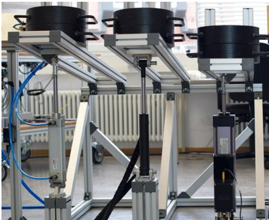
Picture 1: Energy comparison of a pneumatic, hydraulic and electro mechanical actuator (from Exlar).
