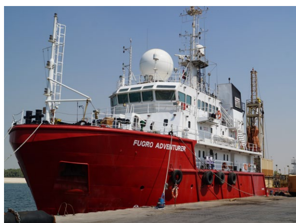
Adventurer dedicated DP2 geotechnical drilling vessel
